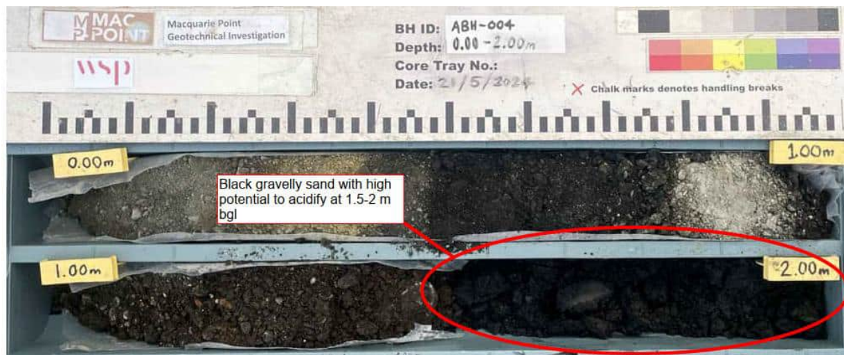
Plate 1 PASS Type 1 - Estuarine material in unsaturated fill (ABH-004 – Core Log at 0 to 2 m bgl) (AECOM, 2025d)
