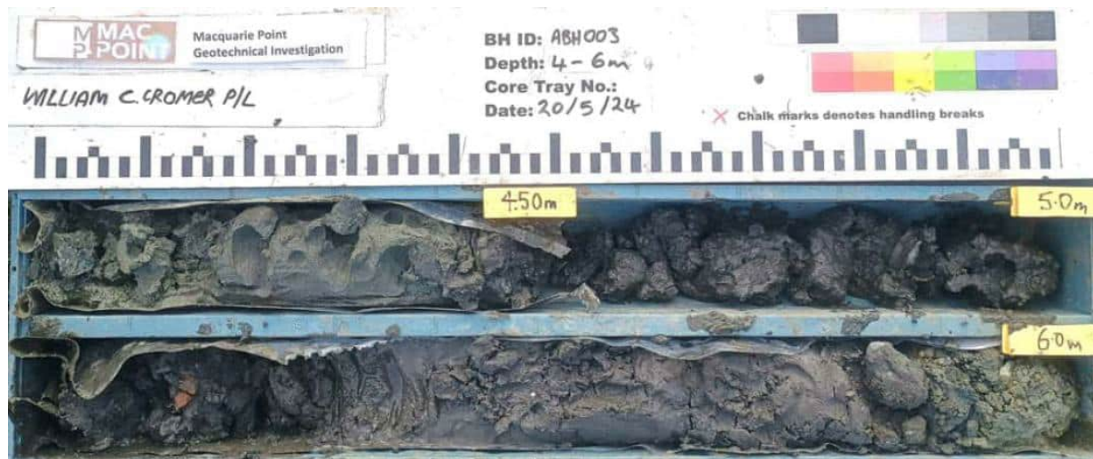
Plate 3 PASS Type 2 and Type 3 - Saturated soil below the water table (ABH-003 - core log 4 to 6 m bgl) (AECOM, 2025d)
