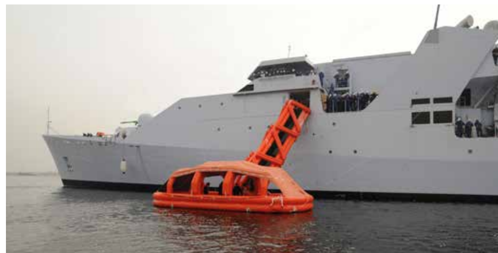
Liferaft Systems Australia Marine Evacuation System deployed from a Royal Netherlands Navy Holland Class OPV.
